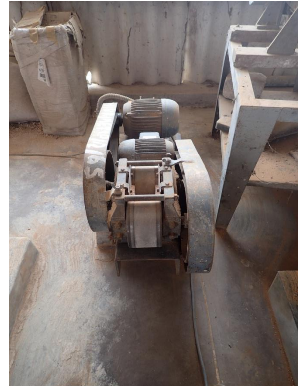
Roller mill for crushing calcinated dolomite of NISIR
