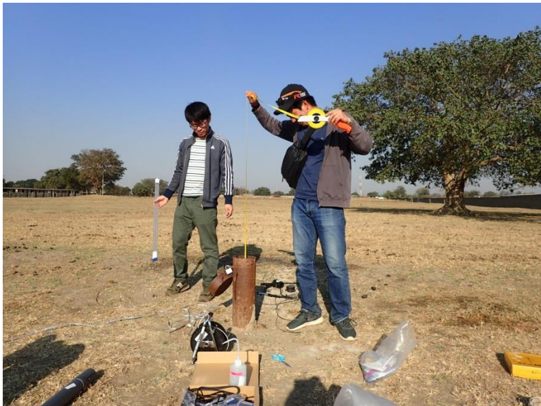
Groundwater sampling by bailer
